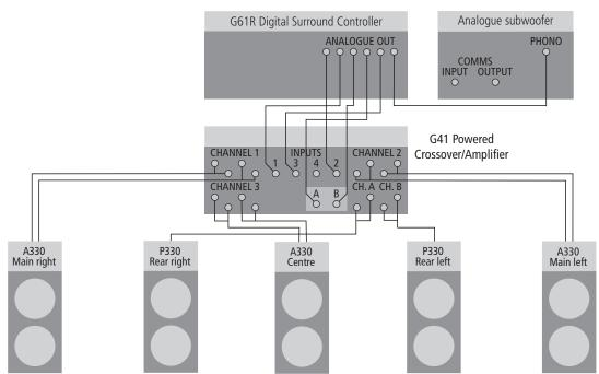
The G61R provides six analogue outputs to allow you to connect to six power amplifiers and passive loudspeakers, or 300 Series Active and Passive Installation Loudspeakers powered by the G41 Active Crossover Amplifier.
