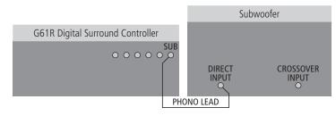
The Meridian SW1600 and SW5500 subwoofers provide both digital and analogue inputs, allowing you to connect them to either the digital or analogue subwoofer outputs of the G61R. The analogue connection must be used if you do not have a digital main speaker.
